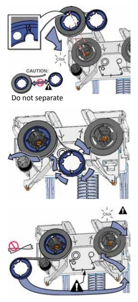
b. Load the topping foil onto the cartridge.
