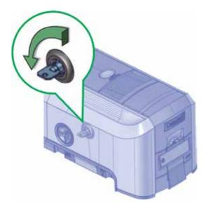
c. Unlock the embosser and remove the indent ribbon and topping foil cartridges.
