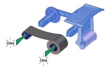
g. Install the print ribbon cartridge in the printer.
