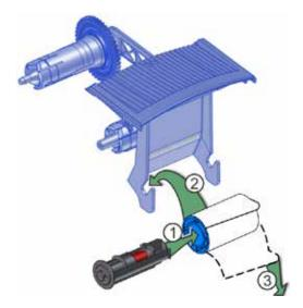
f. If your printer is equipped with the optional printhead, load the print ribbon onto the cartridge.
