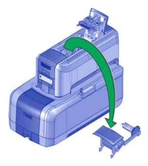
e. Load the cleaning sleeve onto the cartridge.
