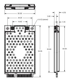
IM11 RFID Reader Module Physical Specifications 50.95 mm long x 30 mm wide x 4.78 mm thick Exceptions to the MiniPCI Express form factor: top side thickness is 2.4 mm (instead of 2.01 mm) and bottom side thickness is 1.35 mm (instead of 1.75 mm).
